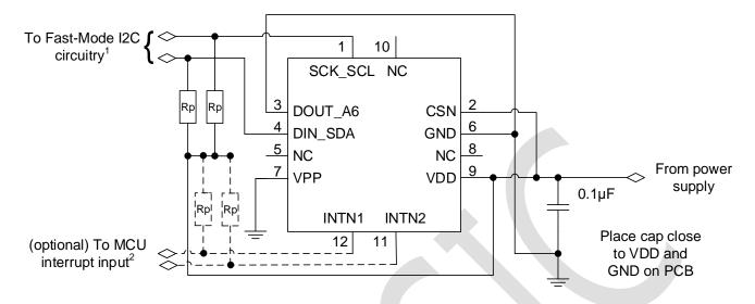
NOTE<sup>1</sup>: Rp are typically  $4.7k\Omega$  pullup resistors to VDDIO, per I2C specification. When VDDIO is powered down, DIN\_SDA and SCK\_SCL will be driven low by internal ESD diodes.
