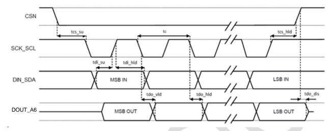
Figure 11. SPI Interface Timing Waveform
