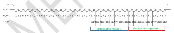
Figure 18. SPI Register Read Cycle - Burst (2 register burst example)
