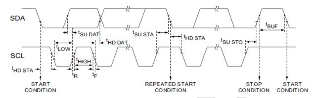
Figure 10. I2C Interface Timing
