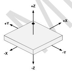
Figure 4. Package Axis Reference
