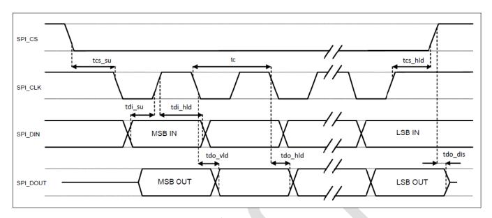
Figure 19. SPI Interface Timing
