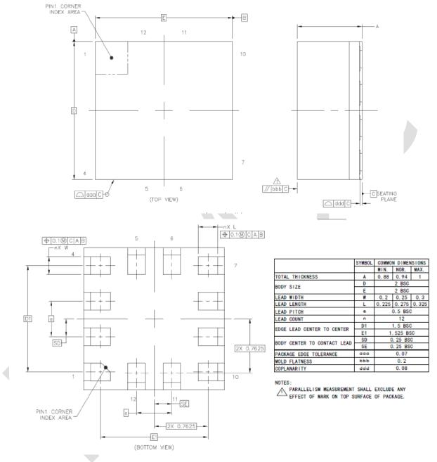
Figure 2. Package Outline and Mechanical Dimensions
