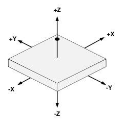
Figure 4. Package Axis Reference
