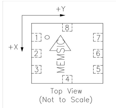
**Note:** The MEMSIC logo’s arrow indicates the -X sensing direction of the device. The +Y sensing direction is rotated 90° away from the +X direction following the right-hand rule. Small circle indicates pin one (1).
