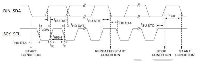
Figure 10. I2C Interface Timing
