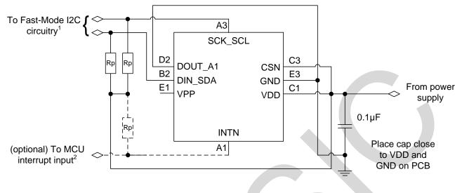
NOTE<sup>1</sup>: Rp are typically 4.7kΩ pullup resistors to VDDIO, per I2C specification. When VDDIO is powered down, DIN\_SDA and SCK\_SCL will be driven low by internal ESD diodes. NOTE<sup>2</sup>: Attach typical 4.7kΩ pullup resistor if INTN is defined as open-drain.
