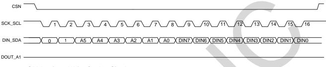
Figure 17. SPI Register Write Cycle - Single
