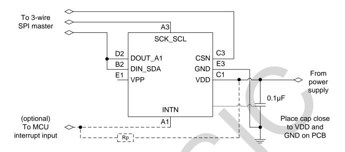
NOTE Rp: Attach typical  $4.7k\Omega$  pullup resistor if INTN is defined as open-drain.
