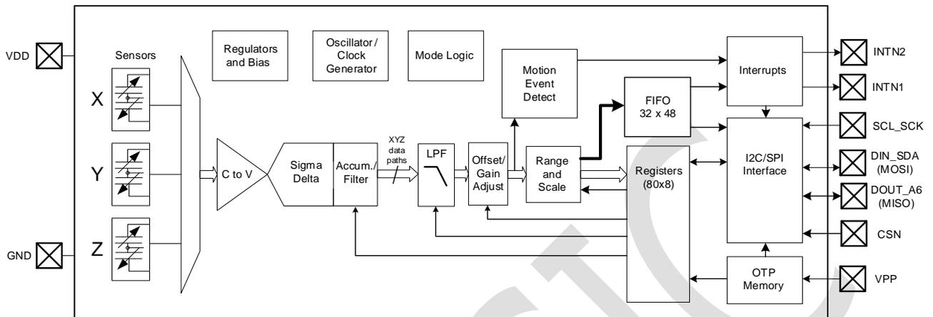
Figure 1. Block Diagram
