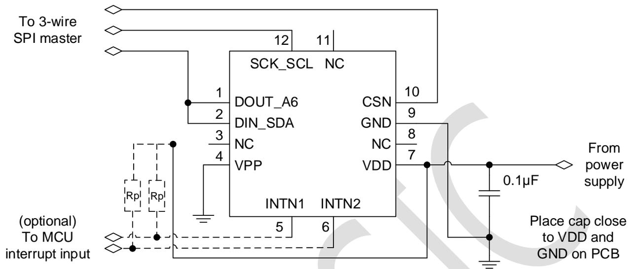
NOTE  $R_p$ : Attach typical  $4.7\text{k}\Omega$  pullup resistor if INTN is defined as open-drain.
