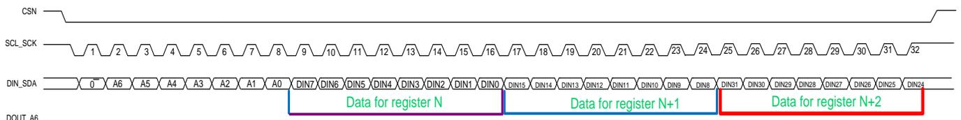
Figure 15. SPI Register Write Cycle - Burst (3-register burst example)
