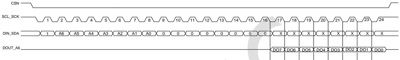
Figure 16. SPI Register Read Cycle - Single
