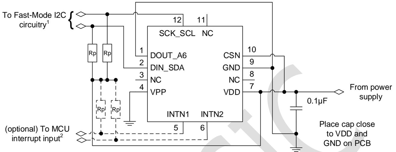
NOTE<sup>1</sup>: Rp are typically 4.7kΩ pullup resistors to VDDIO, per I2C specification. When VDDIO is powered down, DIN\_SDA and SCK\_SCL will be driven low by internal ESD diodes.
