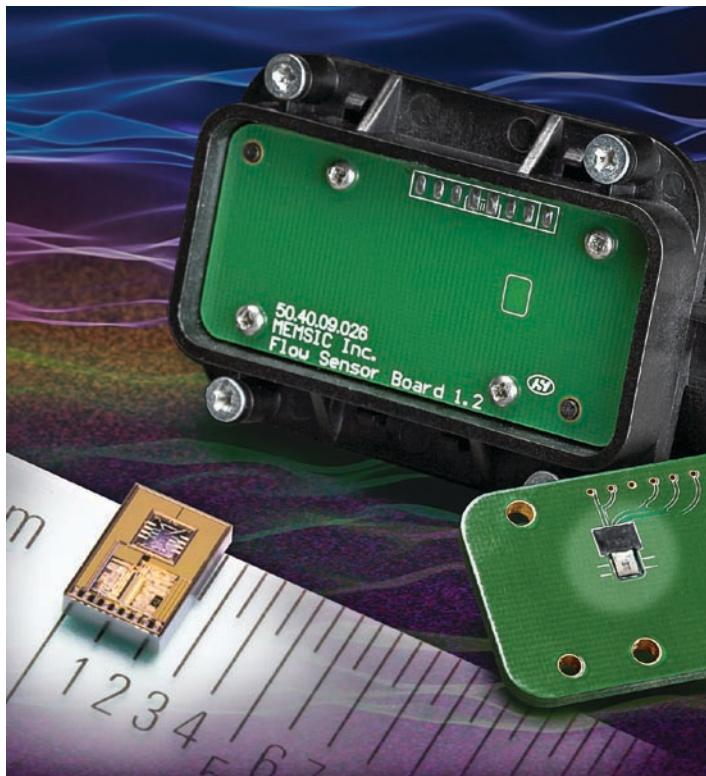
Fig. 1: The MFA1100R thermal gas-flow sensor module integrates the sensing element with on-chip signal-processing and software on a monolithic CMOS process.
