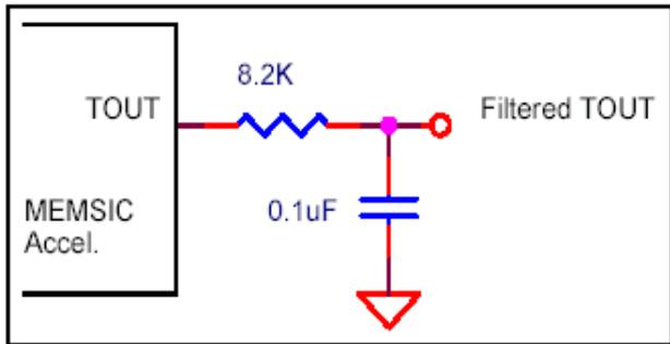
Figure 6: Temperature Output Noise Reduction
