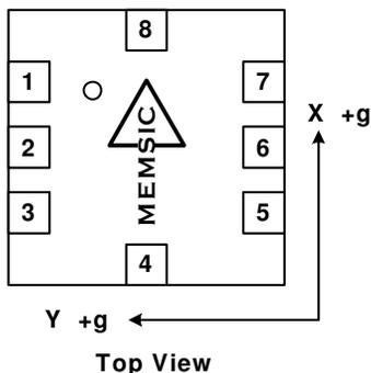
**Note:** The MEMSIC logo's arrow indicates the +X sensing direction of the device. The +Y sensing direction is rotated 90° away from the +X direction following the right-hand rule. Small circle indicates pin one (1).
