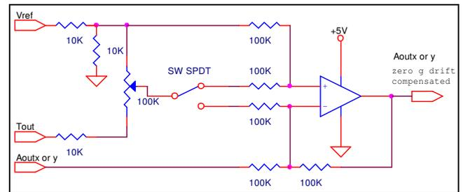
Figure 5: Zero g Offset Temperature Compensation Circuit
